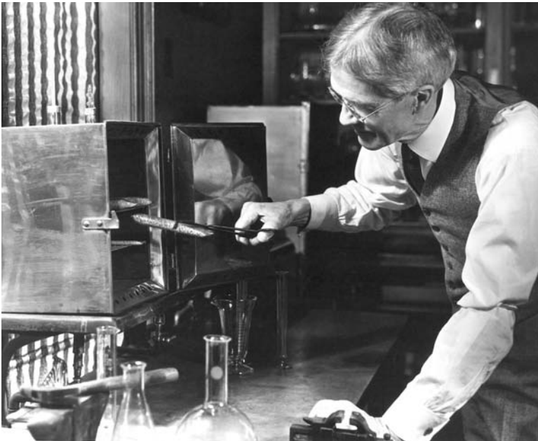
Alexander P. Anderson demonstrates the first experiment, 1902, of the puffing process with rice in sealed tubes being placed in a copper oven. Tower View. 1933
